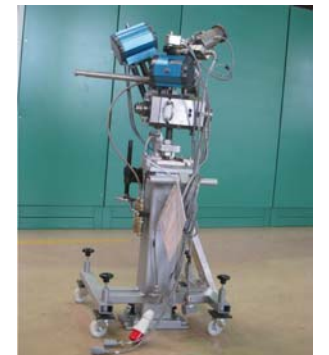
Crosshead: Oil headed/cooled to optimize process conditions for highest foam rates. Floor mounted support, with trolley.
