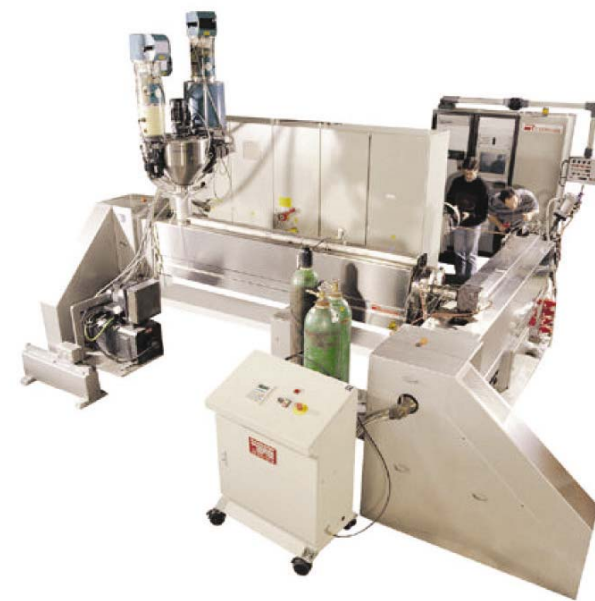
Cascade Extrusion for maximum process stability and highest quality of the dielectric: two separately adjustable processing units provide homogenous melt according to a defined temperature profile, even distribution of nucleating agents and dissolved gas, and a minimum pulsations at the outlet.
